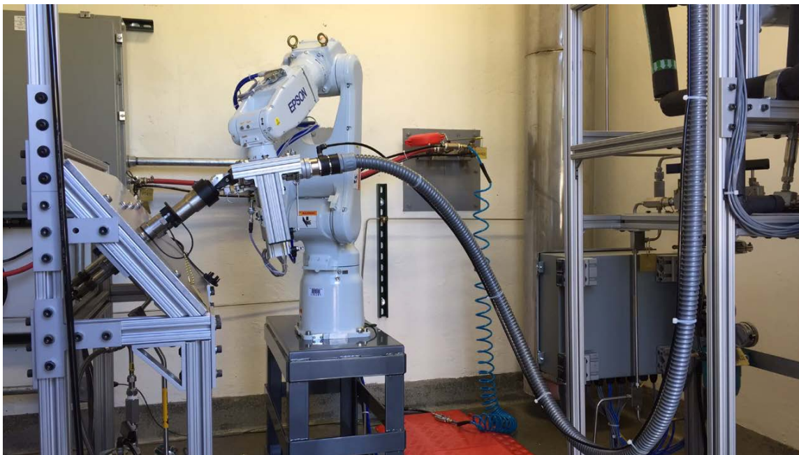
Figure 1. Hose reliability test stand
