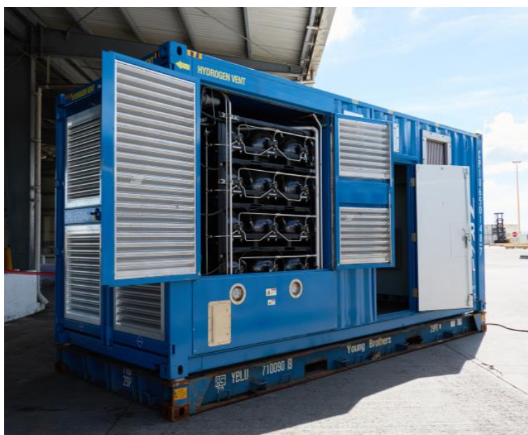
Figure 1. The 100-kW maritime fuel cell generator (MarFC), with integrated hydrogen storage, PEM fuel cell power generation, and power conditioning equipment
