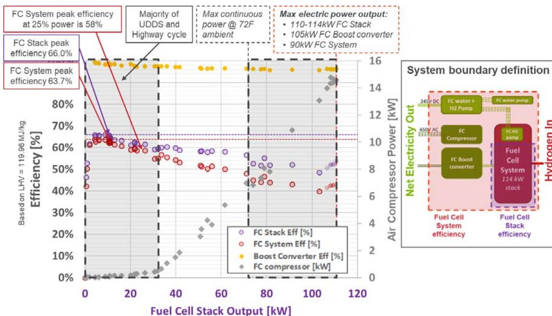
**Figure 3. FC stack and FC system efficiency as a function of electric power output of the stack**
