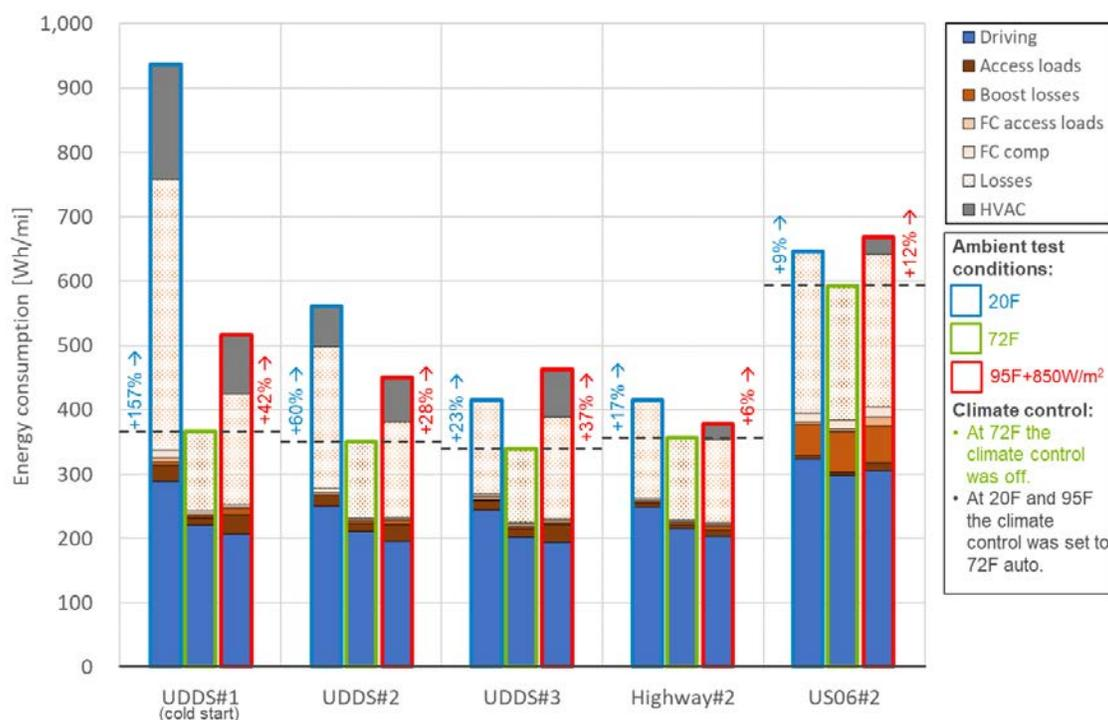
**Figure 4. Hydrogen energy consumption and energy breakdown for different drive cycles across different temperatures**
