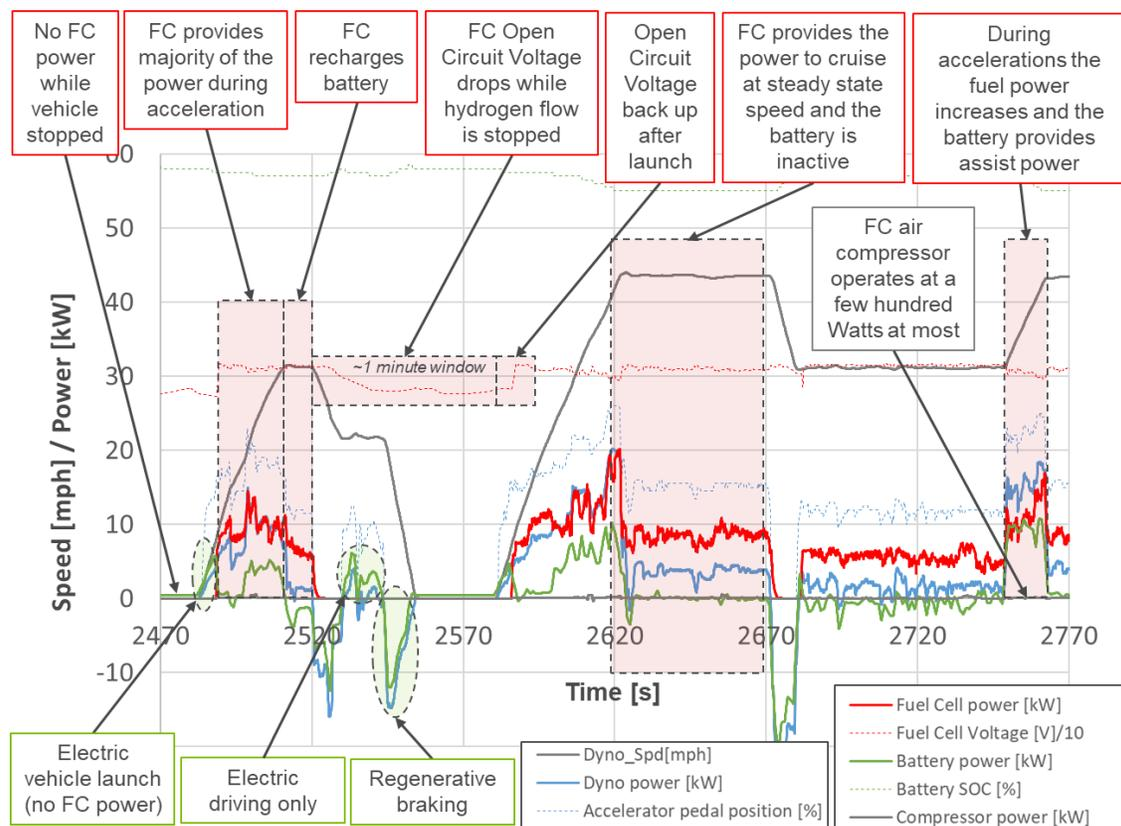
Figure 2. Powertrain and FC system operation in different drive modes on the linear segment drive cycle
