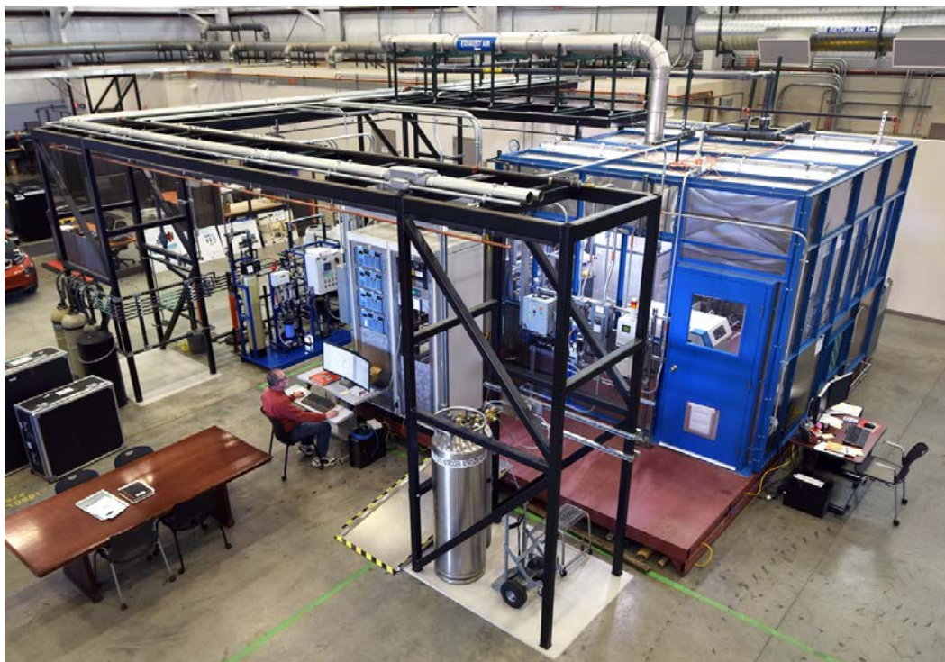
Figure 1. Overview of the 25-kW HTE experiment skid and enclosure within the INL System Integration Laboratory
