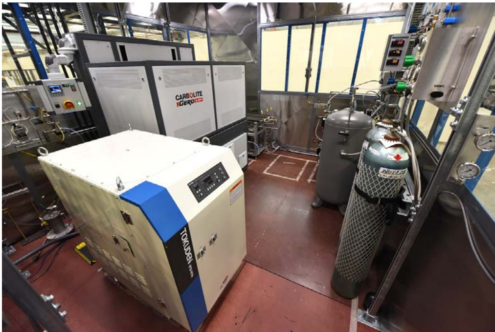
Figure 2. Superheated steam generator and high-temperature furnace in experiment enclosure
