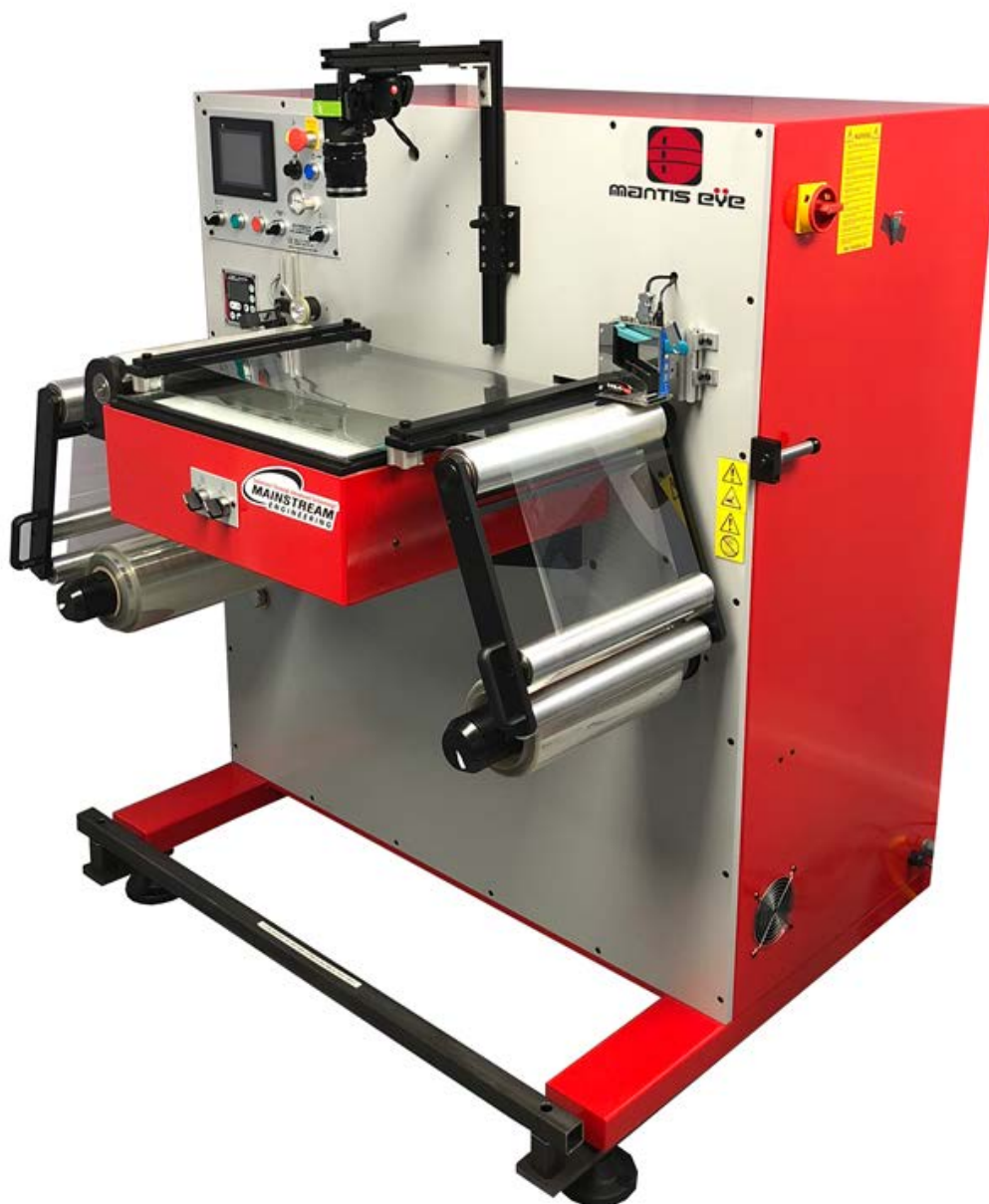
Figure 1. Mainstream's Mantis Eye prototype detector installed on Mainstream's inspection winder
