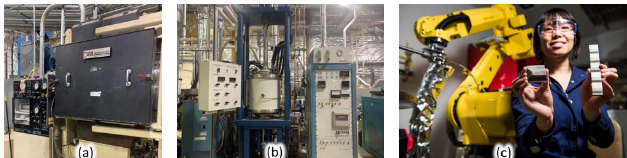
Figure 2. PNNL equipment for coupon fabrication in FY 2020: (a) super plastic forming machine; (b) vacuum hot press; and (c) high-pressure cold spray robotic system
