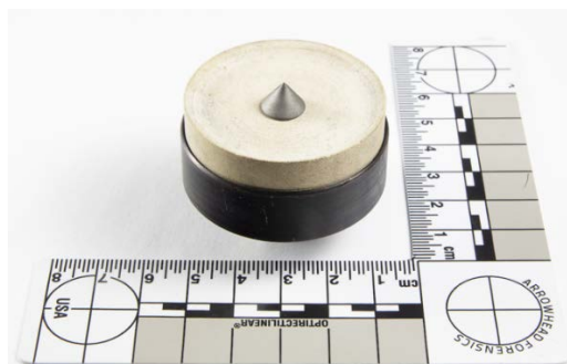
Figure 4. Picture of the new rotating disc made of 100% ceramics
