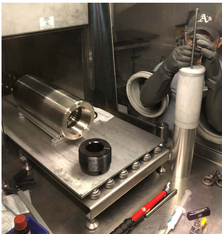
Figure 2. Prepping the inner subassembly to be inserted into the pressure vessel
