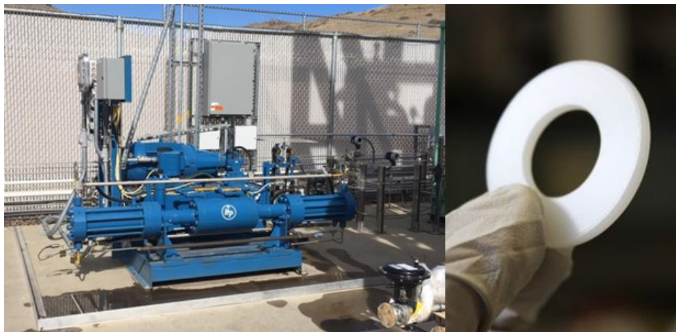
Figure 2. Left: Hydropac hydrogen compressor used to test GVD's PTFE-coated seals at NREL in Golden, Colorado. Right: a representative seal used in a hydrogen compressor.
