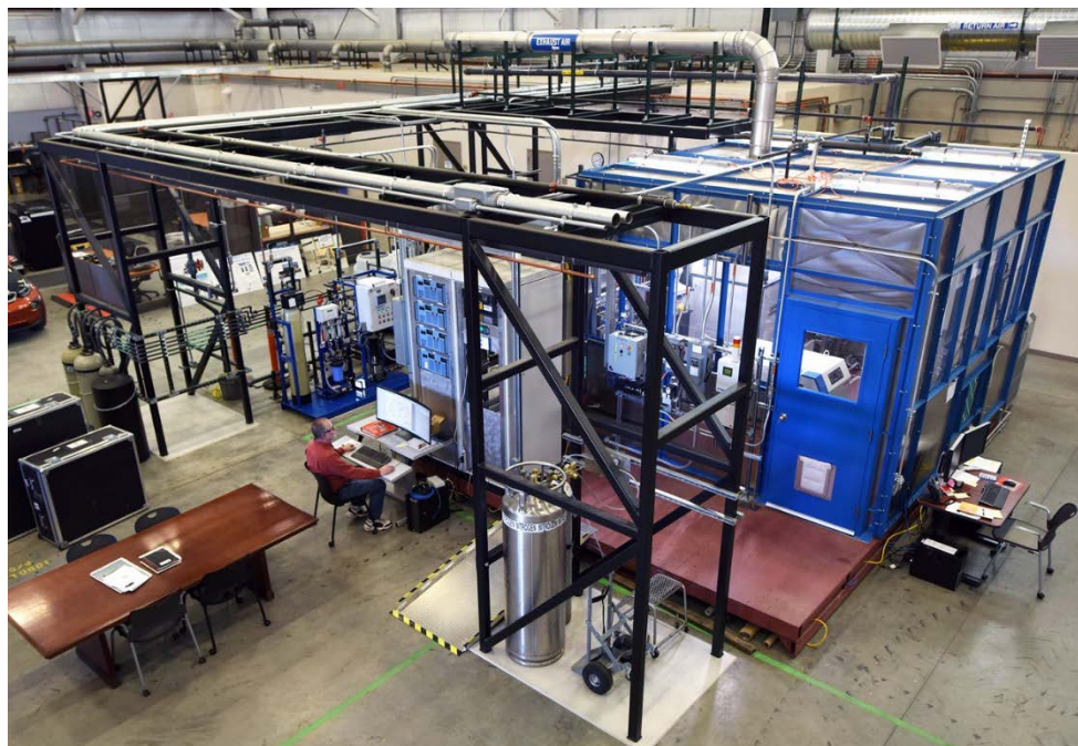
Figure 1. Overview of the 25-kW HTE experiment skid and enclosure within the INL Systems Integration Laboratory.
