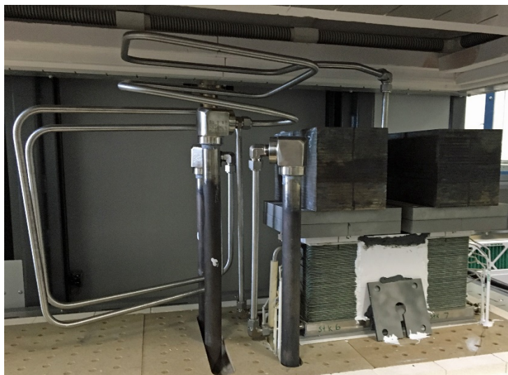
Figure 3. 5-kW stack installation in INL furnace showing coiled process gas inlet lines and dead weights
