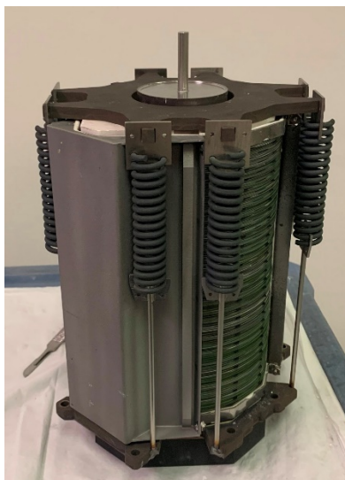
Figure 2. Picture of the 150-cell CSA stack fabricated via an automated manufacturing process
