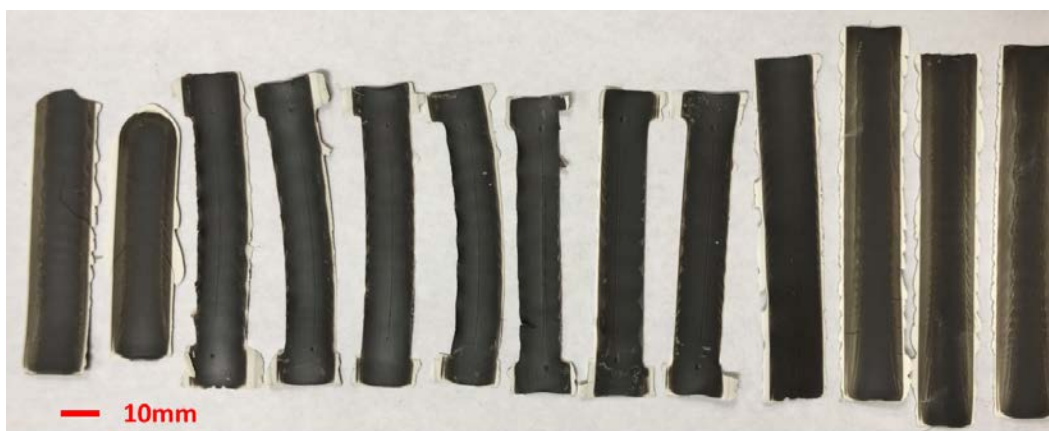
Figure 3. Summary optical photo of half cells fabricated by L3DP
