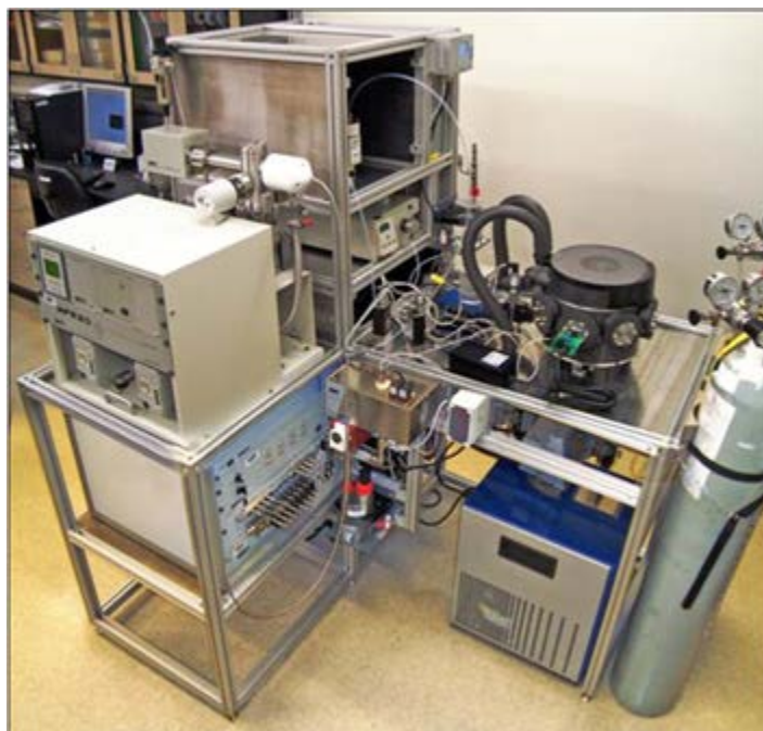
Figure 1. The NREL hydrogen sensor test apparatus
