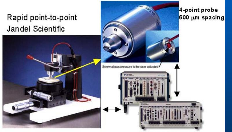
PXI-Based AC Signal Generator and Measurement
