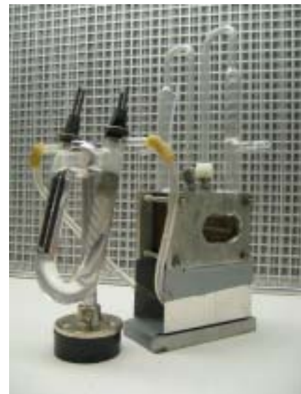
Electrolyzer with fuel cell for safe measurement of in-situ XANES
