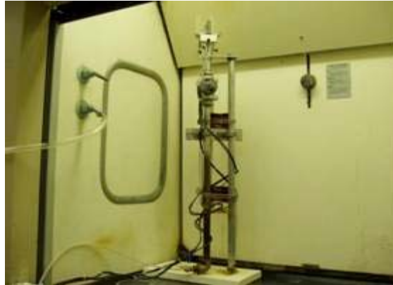
Furnace for Hydrogen Treatment at High Temperature and Safety Equipment
