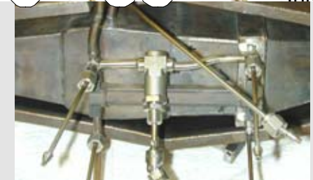
Recuperator Bypass valve
