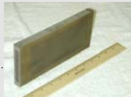
Low-dP steam generator for 50 kWe ATR system.
