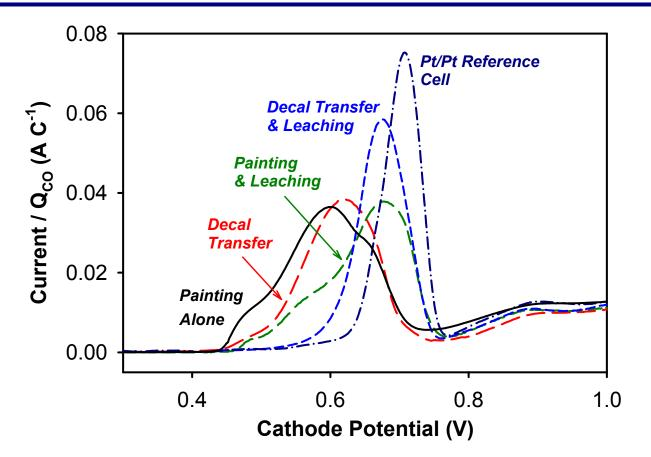
• Virtually Ru-free cathodes observed following removal of loosely-bound Ru in the anode catalyst & better anode curing (after break-in data; no life-tests performed).
