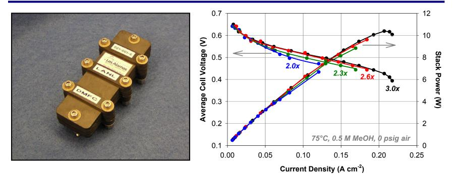
*First test of high specific-power stack: (i) uniform operation of individual cells, (ii) very little sensitivity to the air flow, (iii) anode-limited performance.*
