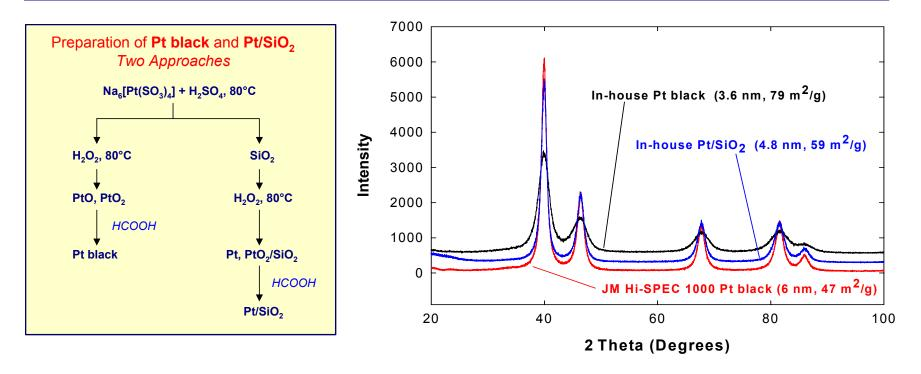
Average particle size reduced from 6 nm (Johnson Matthey's HiSPEC™ 1000, the state-of-the-art Pt black catalyst for DMFCs) to 3.6 nm and 4.8 nm, for Pt black and Pt/SiO<sub>2</sub> catalysts, respectively.
