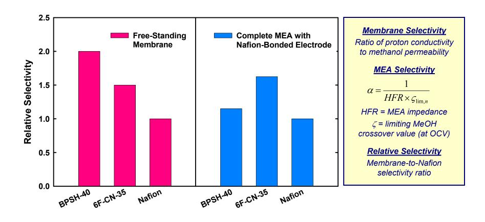
• Expected selectivity gains of BPSH-40 not realized in fuel cell testing.
