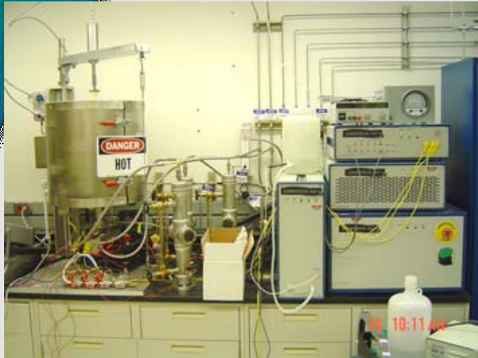
Fuel Cell Test Bed with Furnace, Fuel Source and Test Circuit
