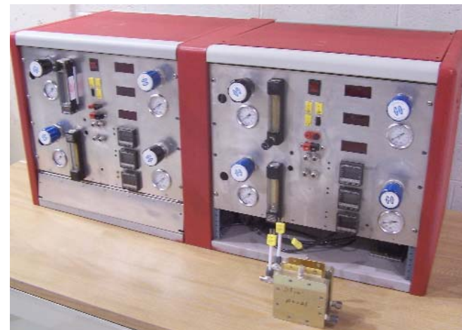
Fuel Cell Test Stations
