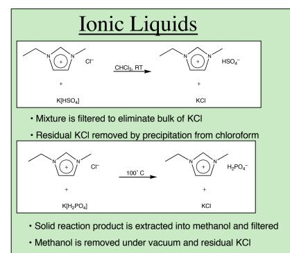
removed by precipitation from CHCl<sub>3</sub>
