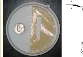
water uptake is high (45%) and this particular membrane is water soluble when doped with acid.
