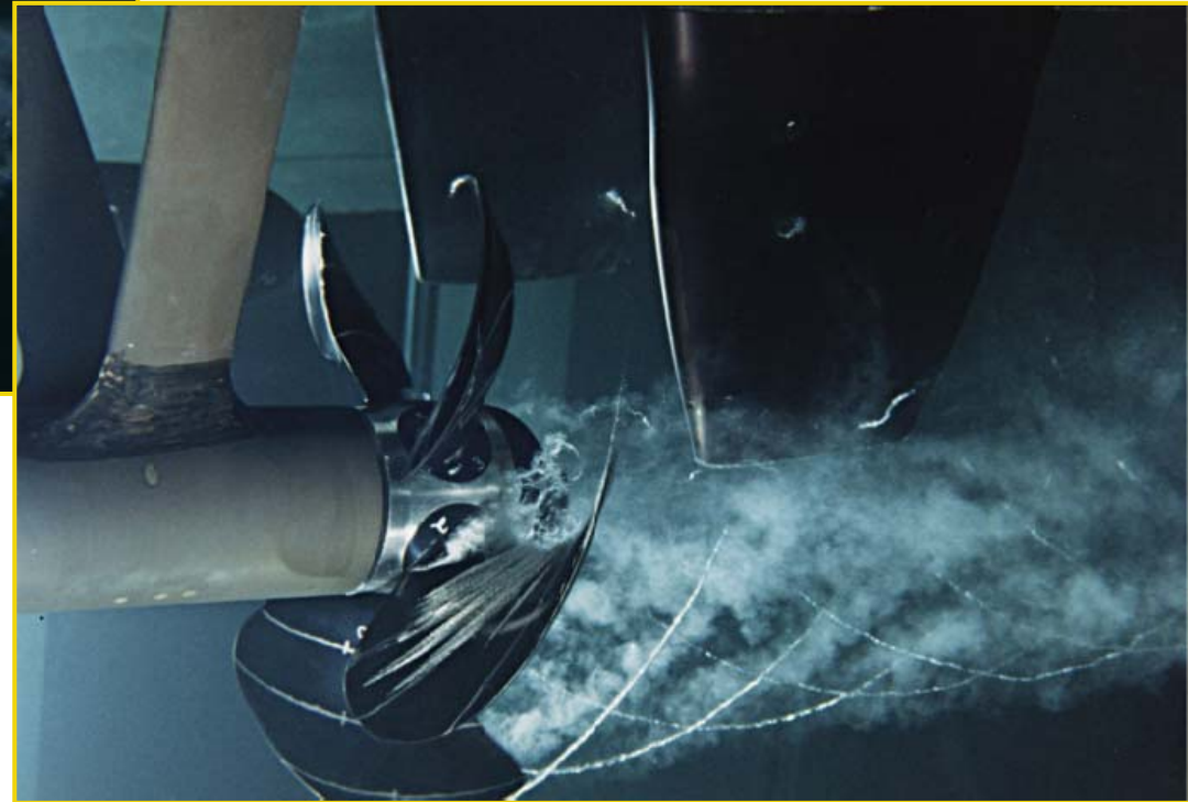
No Rudder Cavitation
