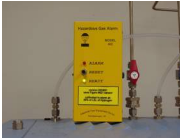
PEM Fuel Cell Dual Station with a Hydrogen Sensor
