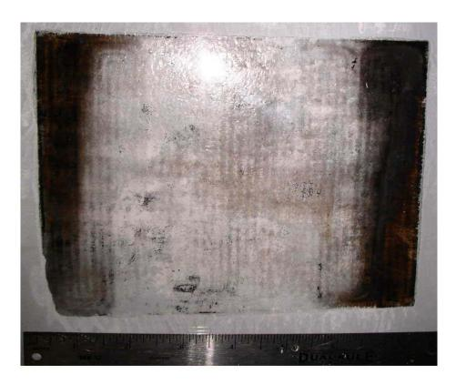
Used NAFION® N112 membrane with catalyst removed, contamination visible at reactant gas inlets on the left and right.
