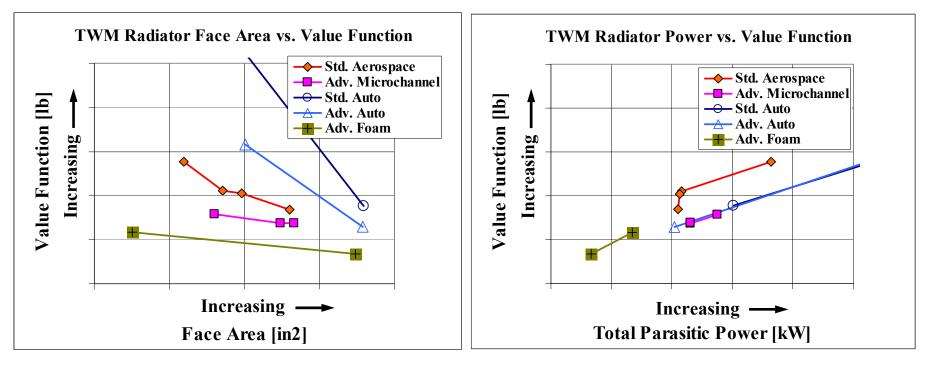
Al foam and microchannel have lowest equivalent weight as face area is reduced Al foam has smallest power requirements Able to meet power targets
