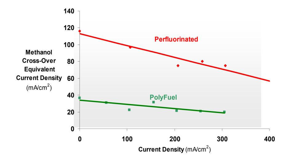
Note: Standard PolyFuel Active Test Cell Conditions used
