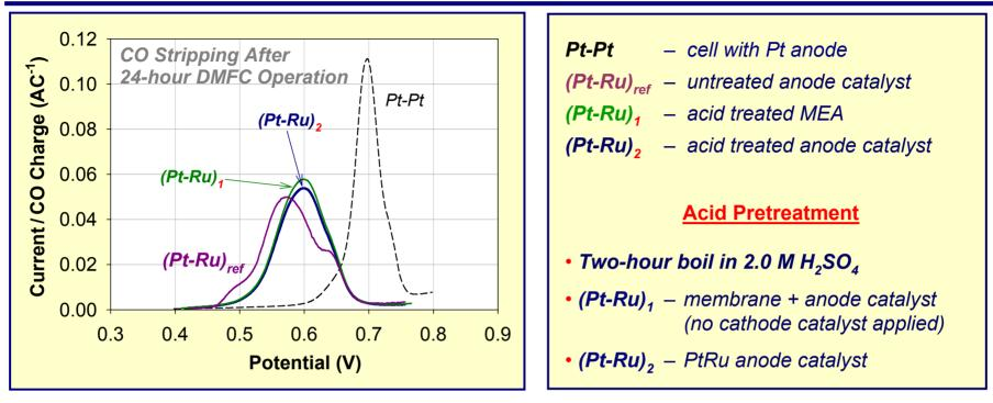
**HIGHLIGHT:** Developed <u>four methods</u> for minimizing Ru crossover; negative shift in CO stripping peak potential reduced by 30–130 mV.
