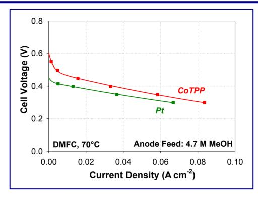
HIGHLIGHT: In cells with relatively high MeOH anode concentration, nonprecious metal CoTPP catalyst easily outperforms the stat-of-the-art Pt black catalyst (2 mg cm<sup>2</sup> loading used with both cathode catalysts)
