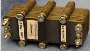
High-power density DMFC stack developed at LANL, integrated by Mesoscopic Devices into 20 W prototype portable power system for the US Government
