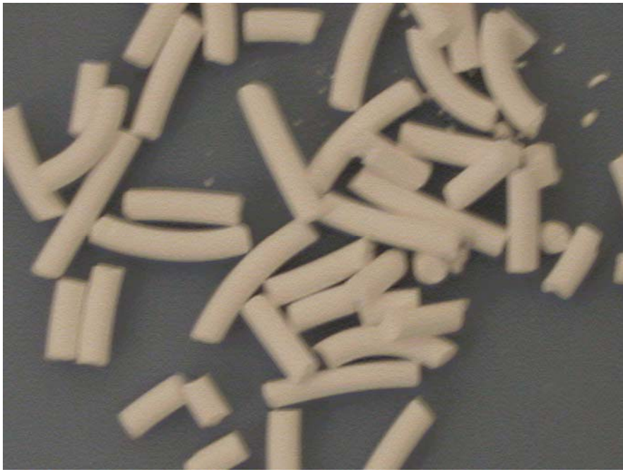
Extrudate B, after 523 cycles
