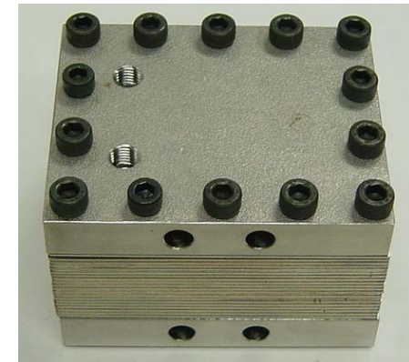
Assembled Module (25 stacks) (77 X 64 X 54 mm)
