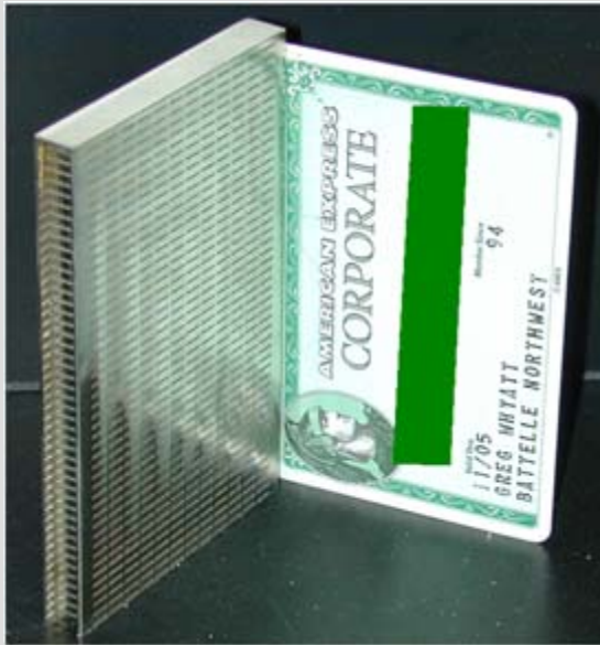
Reforming Reactor Panel
