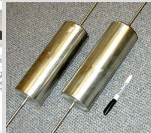
WGS Reactor (Fe-Cr catalyst)
