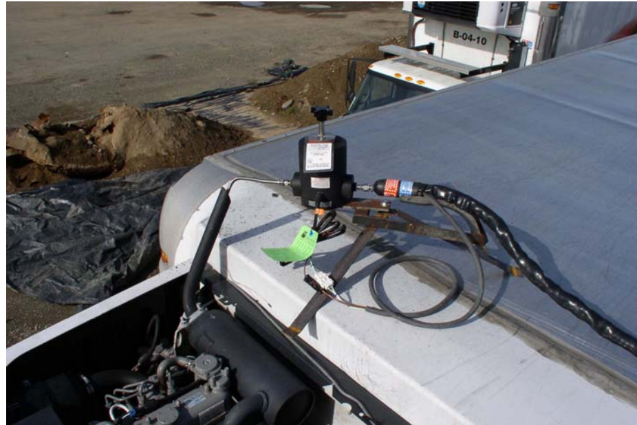
Emissions sampler with exhaust system of the box truck TRU.
