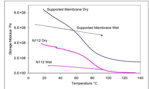
**Dynamic Mechanical Analysis** (DMA) shows the modulus of the novel supported membrane is ~10 X higher than the N112 membrane.
