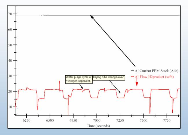
70 A stack current for 30 minutes shows hydrogen product flow rate fluctuations due to internal water and drier management. The testing shows the variability in hydrogen production for this specific model.
