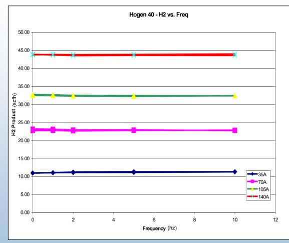
These results show that there is no effect of large DC ripple on hydrogen production.
