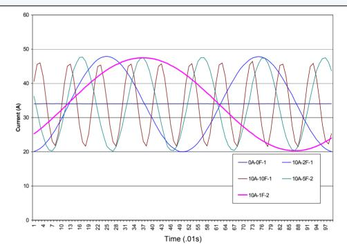
Sample current waveforms used to characterize stack frequency response
