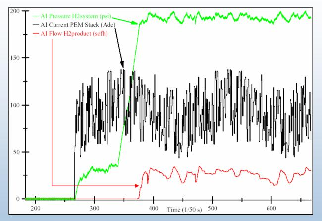
This graph show the hydrogen output and pressures for the simulated wind turbine inputs.
