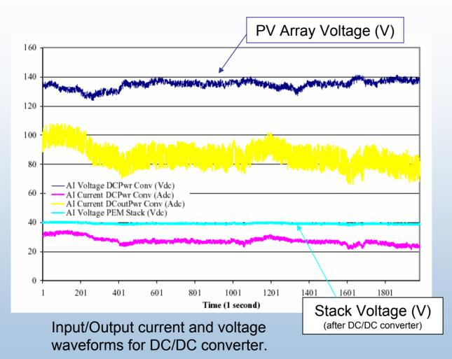
This data shows the functionality of the current DC/DC converter when testing with the PV array.
