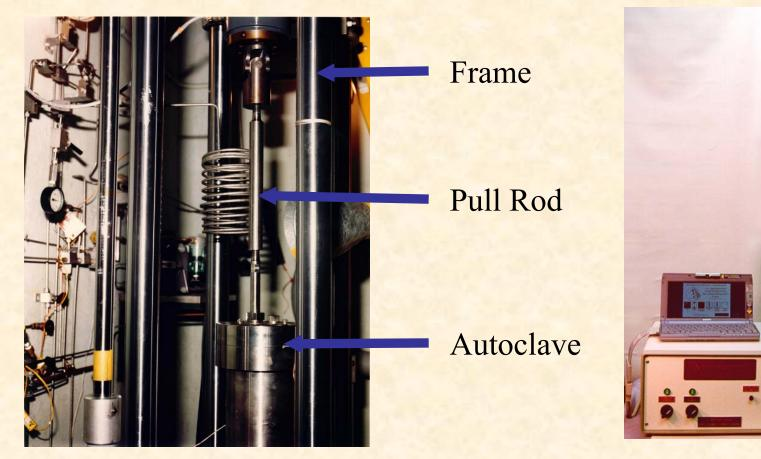
System that will be reassembled at ORNL for mechanical testing at hydrogen pressures upto 5000 psi
