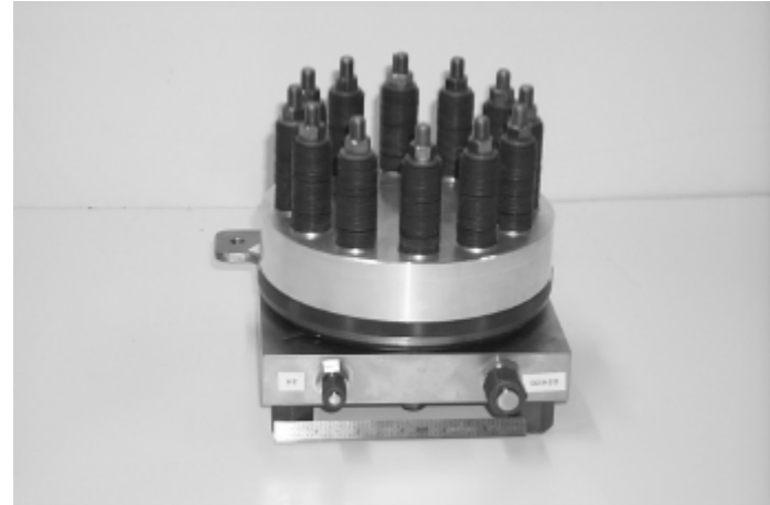
Modified PEM Water Electrolyzer (84 cm 2 active cell area)
