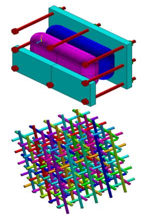
**Conformable pressure vessels** efficiently use available space in the vehicle, increasing truck hydrogen delivery capacity
