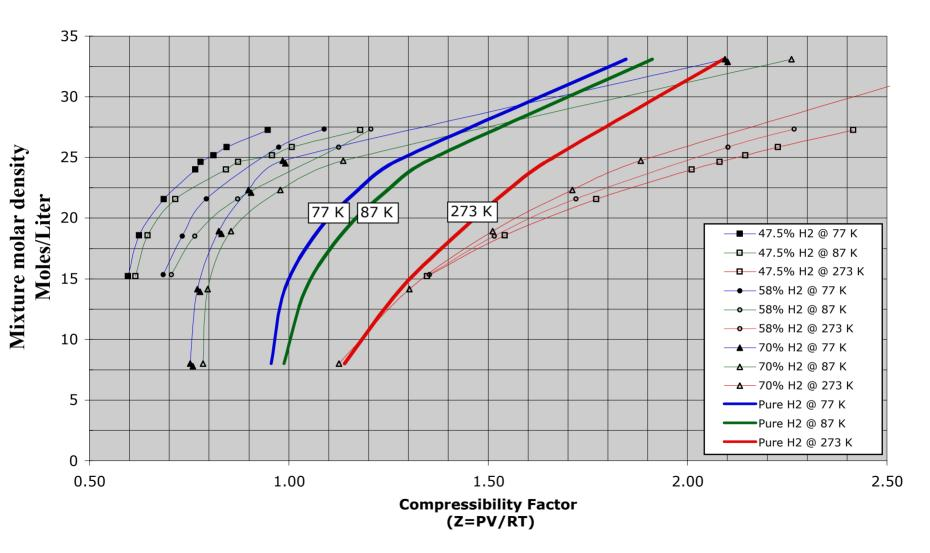
Cooling hydrogen makes it safer: energy release during a sudden failure is a weak function of pressure but a strong function of temperature
