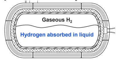
Hydrogen absorbed in liquid nitrogen is safe, easy to dispense, light and compact
