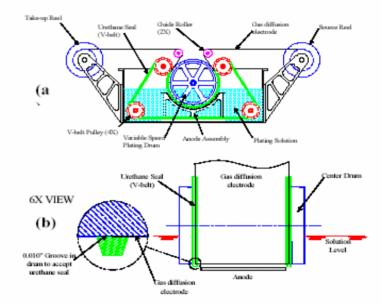
Figure 1: (a) cross-sectional view of the entire reel-toreel apparatus for electrodeposition of platinum onto a gas diffusion electrode; (b) close up of the gas diffusion electrode on the drum, and urethane seal.
