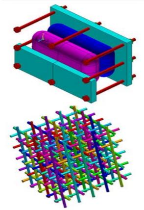
**Conformable containers** efficiently use available space in the vehicle. **Ribs and struts** provide heat transfer paths for efficient thermal management
