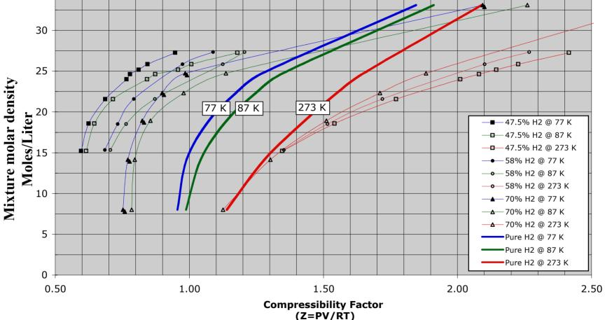
Thick lines are for pure hydrogen and thin lines are for mixtures of hydrogen and nitrogen. At ice temperature (273 K), the compressibility factor (and therefore the volume) is higher for the mixture than for the pure H<sub>2</sub> because no absorption occurs. At LN<sub>2</sub> temperatures, DOF H<sub>2</sub> Program Annual Review, 5-24-2005 considerable absorption occurs, and the mixtures are more compact than the pure H<sub>2</sub>
