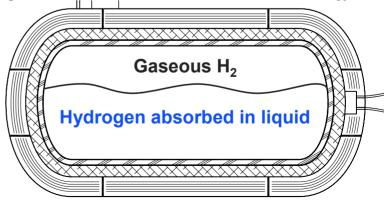
Hydrogen absorbed in liquid nitrogen is safe, easy to dispense, light<sub>D</sub>and<sub>CO</sub>compact<sub>W, 5-24-2005</sub>
