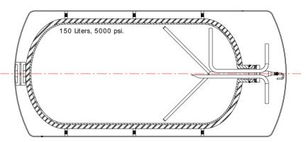
**Insulated pressure vessels** are needed for cryogenic operation with low evaporative losses. **Supercritical hydrogen** (p~5000 psi, T≤50 K) has the potential to meet the 2015 DOE goals
