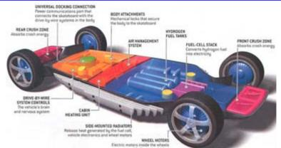
**Compressed:** develop containers for very high pressure (10,000 psi) and moderate temperature (up to 100°C)
