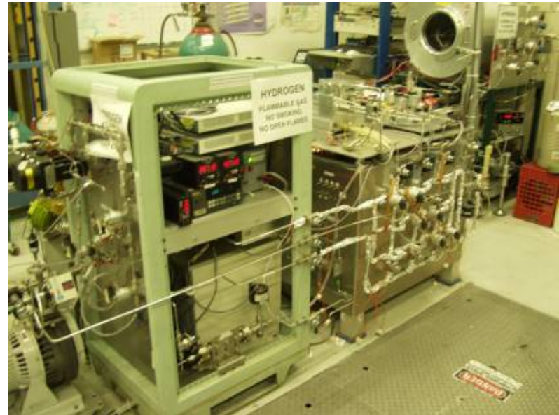
JPL Hydride activation and cycling test station
