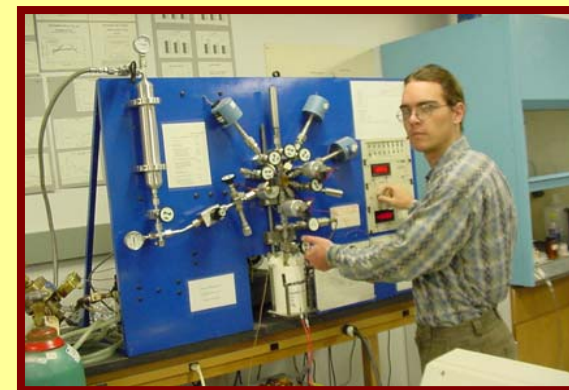
Fully Automated Sievert's Apparatus at UNR to be Modified for Thermal Cycling
