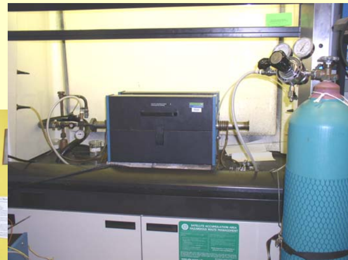
Tube furnace with controlled atmosphere for sample synthesis
