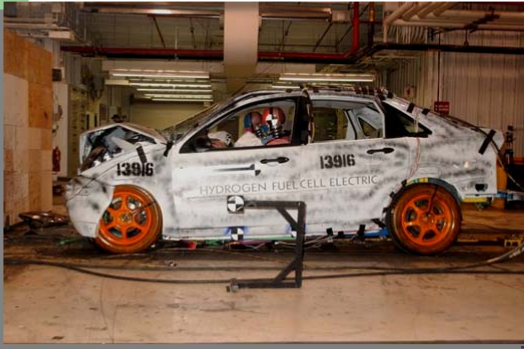
90° 30 MPH Front Fixed Barrier Impact
