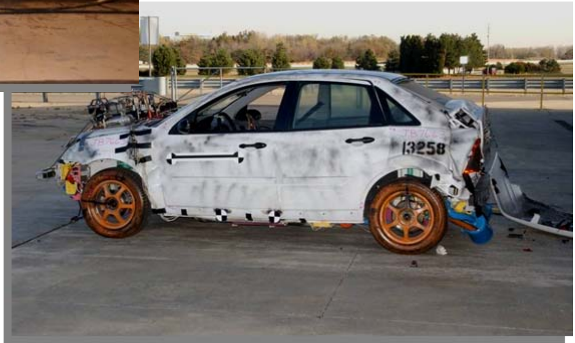
90° 30 MPH Rear Moving Barrier Impact
