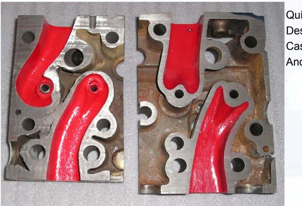
Quiescent Port Designed, Cast, machined And Tested
