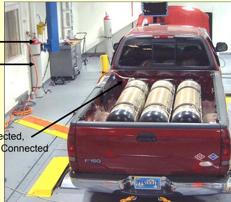
Off-Board Fueling of the Hythane Truck
