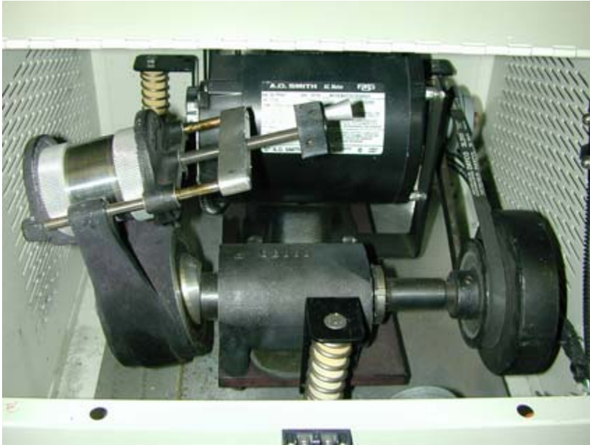
SPEX: high energy; control by balls-to-material mass ratio
