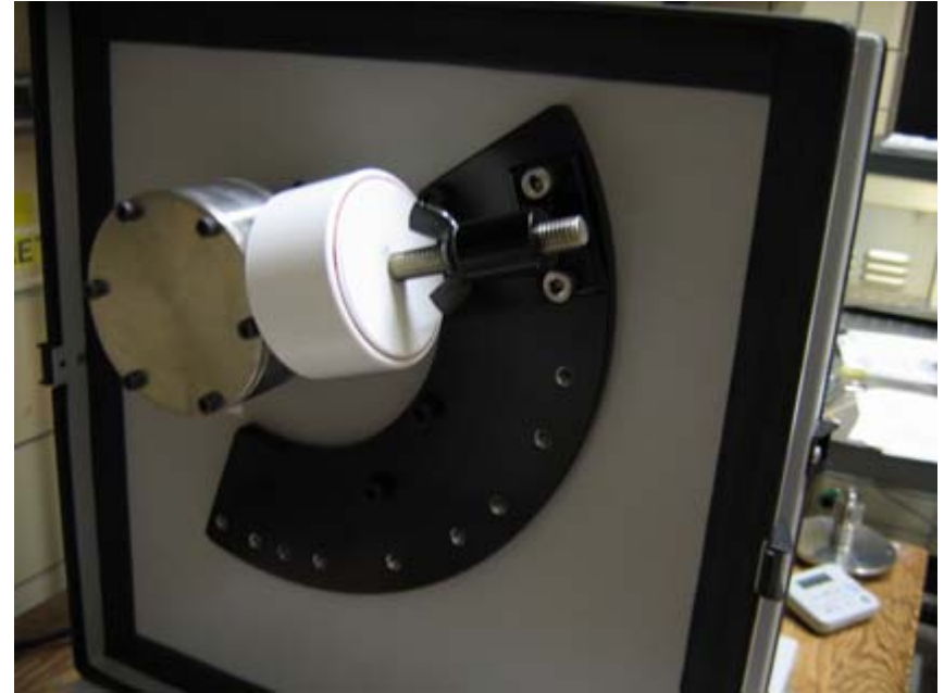
Magnetic: variable energy; control by rpm and positioning of the magnets
