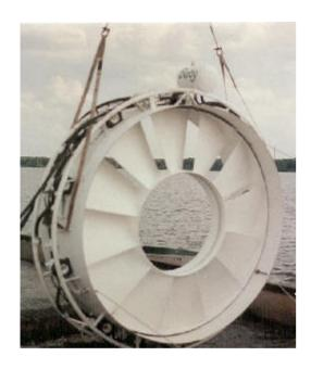
NAVSEA-Carderock and FHPL will test and refine the FHPL innovative open center turbine unit and mooring assembly.
