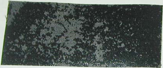
Exterior gas diffusion layers with electrode catalyst removed
