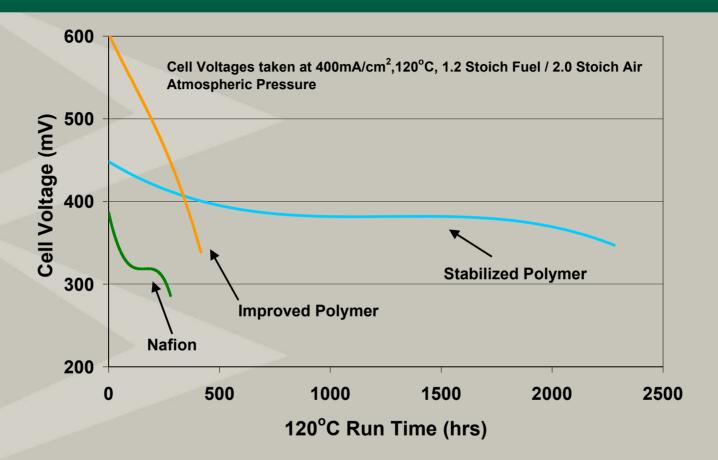
The improved/stabilized polymers show significant increase in cell life at 120°C, ~35% RH
