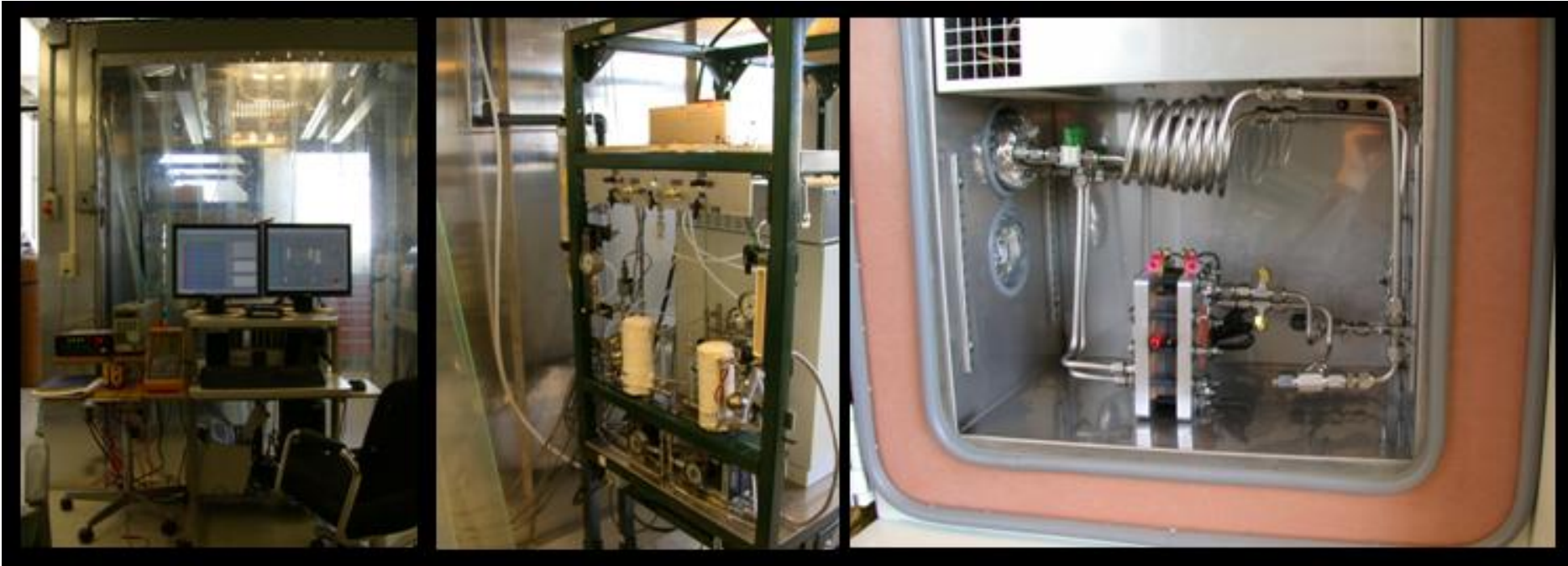
Fuel cell test apparatus. Walk-in hood, test stand, and chamber (from left to right)
