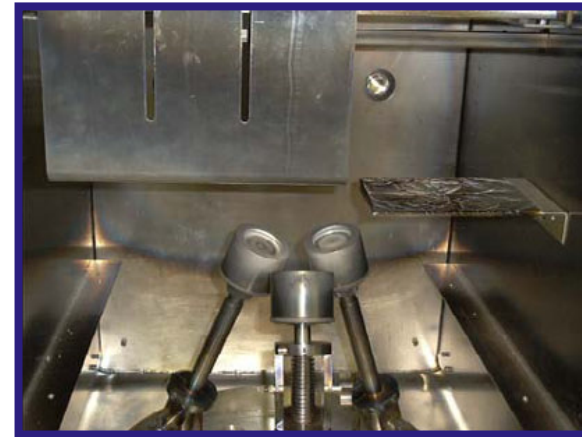
Sputter Chamber with Multiple Targets
